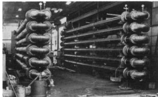
Shop View, Stand of 12 Pipes 8' ID x 42' Lg., Steel Construction. Part of Order for 7 Stands, Dewaxing Lube Oil.
